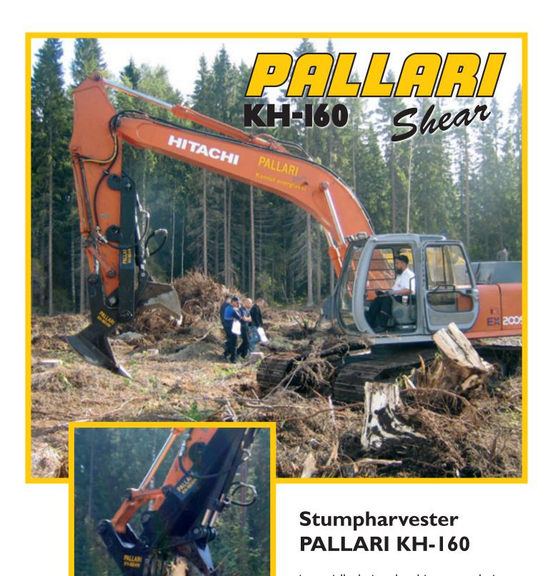
is specially designed multi-purpose device for hydraulic excavators to break up, loosen and take apart all kinds of stumps and roots. Stumpharvester is used for reducing size of all kinds of soft (wooden) recyclable materials.
